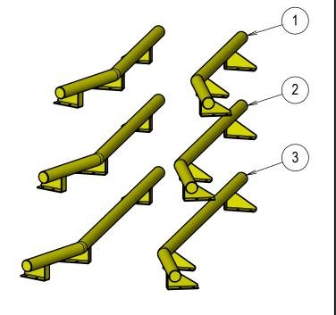
MATERIAL: 4.5"OD x 1/4" WALL STEEL TUBE FINISH: POWDER COATED GOLDEN YELLOW
