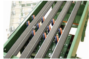
30° Skewed Wheel Diverter (single direction)
