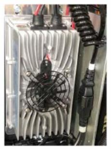
For PSE26N SL the charger with current 25A is used The standard charging time is 2.5 hours
