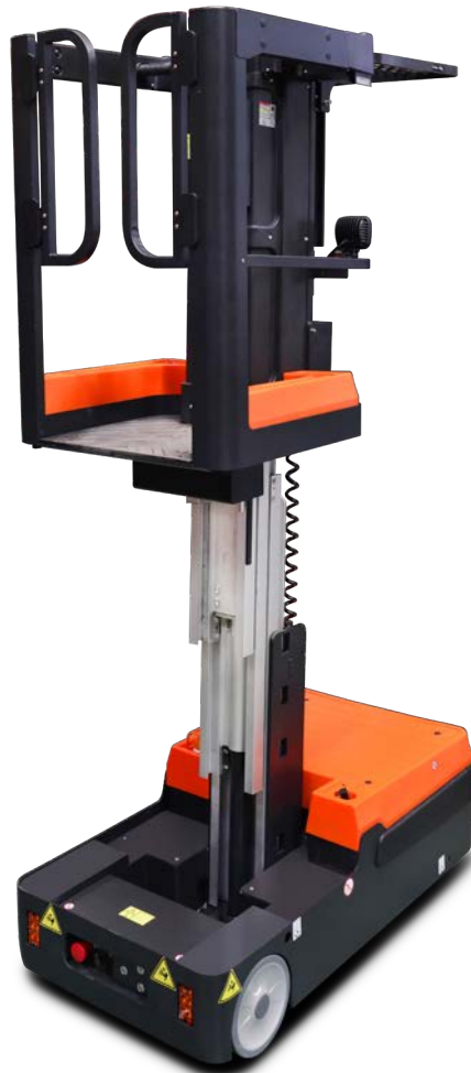
Travel speed 2mph Lifting height between 19.6-59 inches
