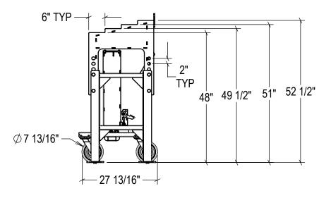
UNIT SHOWN WITH THE STEPPED SUPPORT MOUNTED IN THE HIGHEST POSITION.
