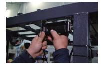
Step 5. With the wire next to the post, adhere light near the backpost of the overhead guard.
