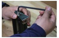
Step 3. Tighten bolt with 3/16" allen wrench.
