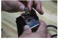
Step 2. Place the mounting bracket over the hole and insert short bolt into the bracket with a washer.
