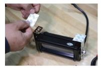
Step 4. Stick 2-way tape on feet of brackets.
