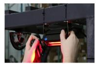
Step 10. Tighten bolts on both sides of the light to secure position.
