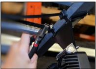
Step 7. Holding bracket in position, tighten both tie straps (if ordered) using pliers for final tightening.
