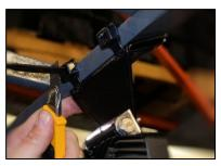
Step 8. Trim excess of both tie straps (if ordered) and ensure any sharp burrs/edges are removed.
